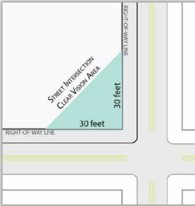
Figure 7-3 Street Intersection Clear Vision Area
